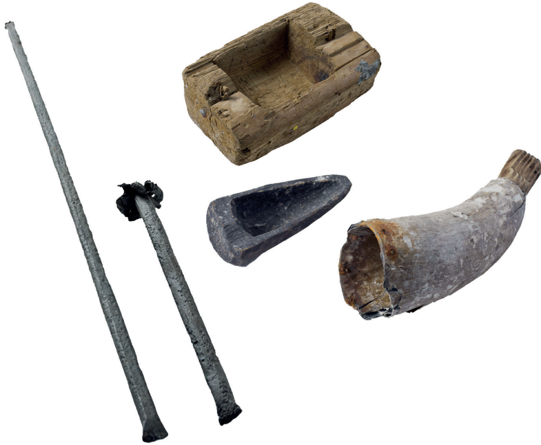
Fig. 1: Brixlegg, Austria, Early Modern Times Fahlore-mining, blaster's hewer tool equipment, consisting of a drilling set, a powder horn, a blaster's loam hod and a powder filling hod
